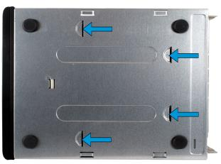
Re-attach the screws on the back of the chassis to secure the motherboard tray in place.
