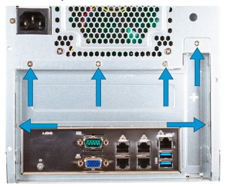
Very carefully pull the tray out of the back of the system. Continously check that no wires are being pulled or caught on other components inside the system.
